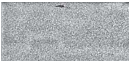
Figure 8. A difference image shows luminance deviations relative to a computed reference image. The location of the mura is highlighted.
