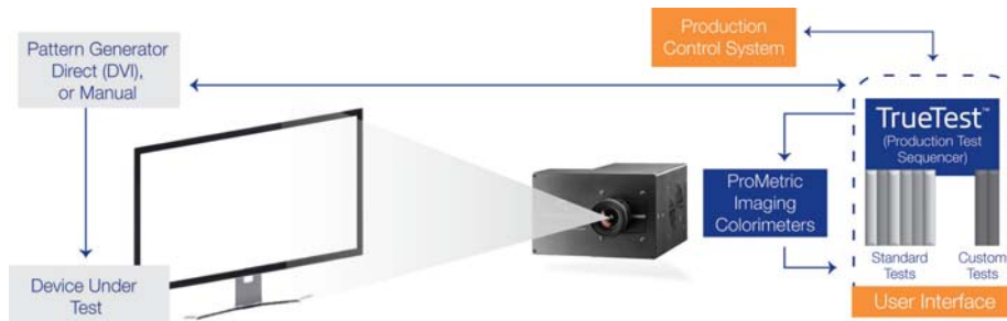
Figure 1. FPD AOI test set-up with an imaging colorimeter under automated software control.
