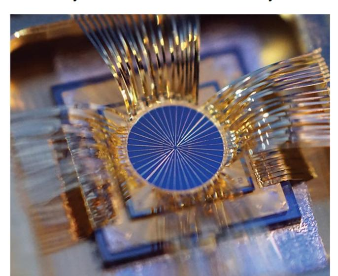
Can diode lasers offer high power — and a good beam profile? Photonic-crystal surface-emitting lasers achieve these qualities and show promise for numerous applications.
