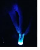
Researchers created light-emitting carbon dots via solvothermal synthesis, where waste was placed into a solvent under pressure and high temperature for 30 to 90 minutes. In this case, the raw materials were soft drinks and pieces of bread and tortilla.
