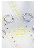
Brillouin scattering-induced transparency (BSIT) permits light to travel in one direction along the fiber while light traveling in the other direction is strongly absorbed.
